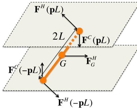
**Figure 1:** A suspended confined fibre is modelled as a rigid dumbbell on which act hydrodynamic ( $\mathbf{F}^H$ ) and contact ( $\mathbf{F}^C$ ) forces.
