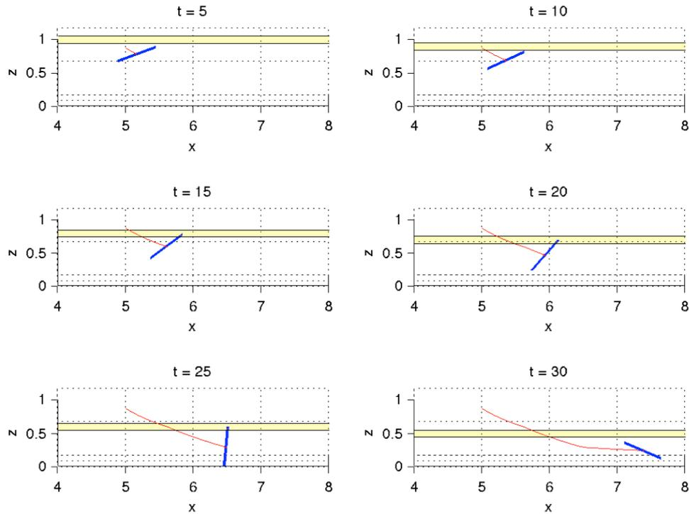
**Figure 2:** Evolution of the position and orientation of a short fibre immersed in a squeeze flow and interacting with the upper gap wall.
